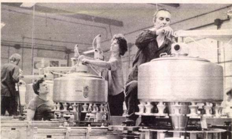
Machines filling cans with peas and French beans
